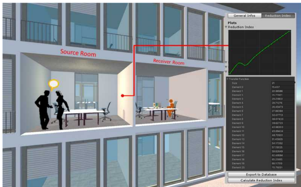
Figure 6.10: An example of predicted sound reduction index ( R' ) for the partition (main separating element) between the adjacent rooms in VBA
