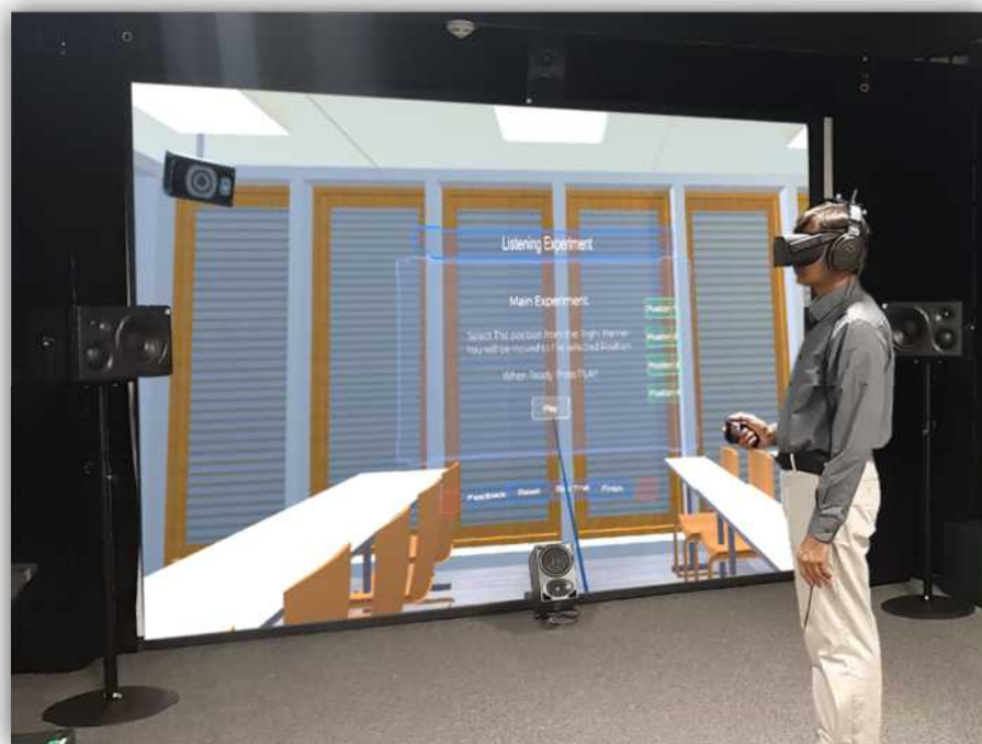
Figure 7.11: HMD view point of the virtual receiving classroom and the experimental setup in VR environment
