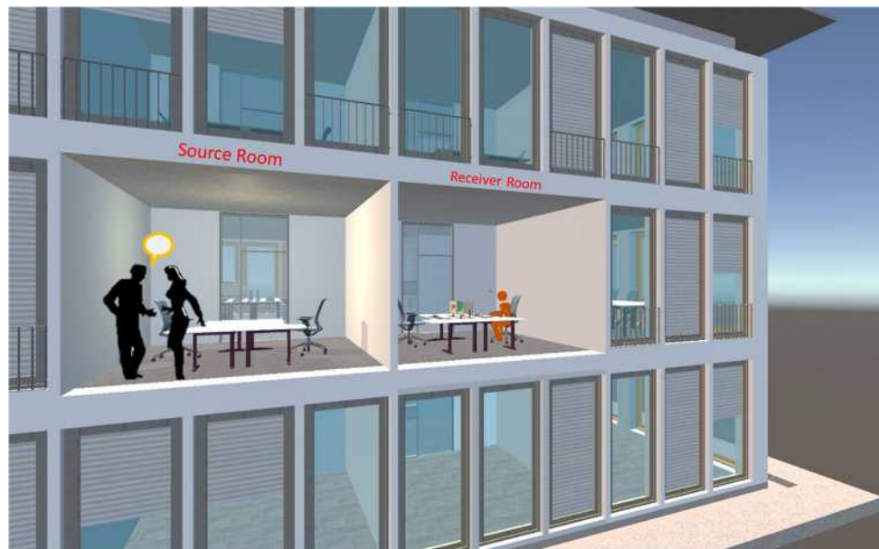
Figure 7.2: Source and receiving room: Office situation in receiving room with work desks and computer screen and persons talking in source room
