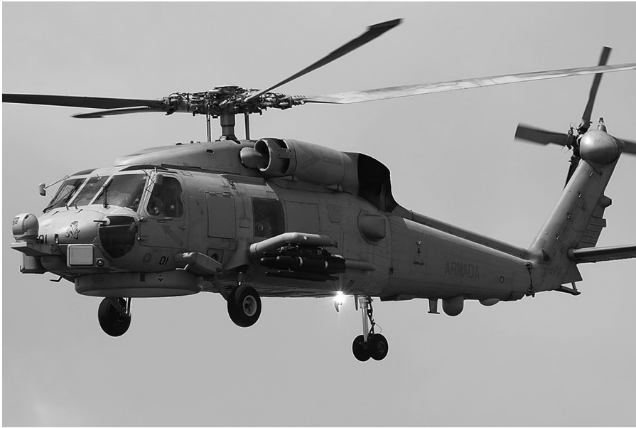
Figure 2.4 An SH-60B in flight (Curimedia 2012). The FLIR system is the spherical module on the nose of the aircraft
