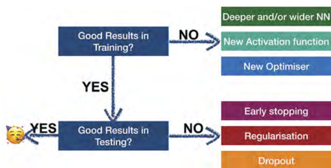
FIGURE 40.4 Tips on tuning the neural network for better model prediction performance.
