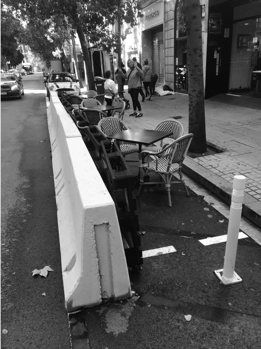
FIGURE 5.8 Barcelona: use of the New Jersey barrier to restructure parking spaces for leisure activities.
