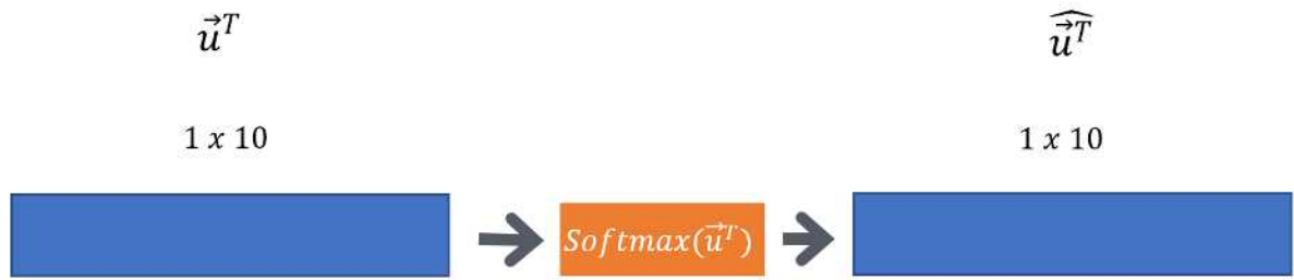
Figure 123: Calculation of the prediction vector \widehat{\vec{u}}^T
