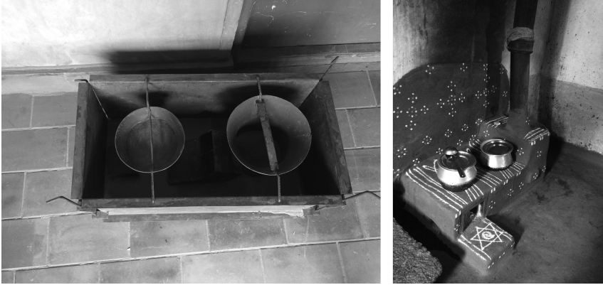
Figure 7.1 Cook stove mould (left), finished mud stove (right). Source: Authors' field photographs.
