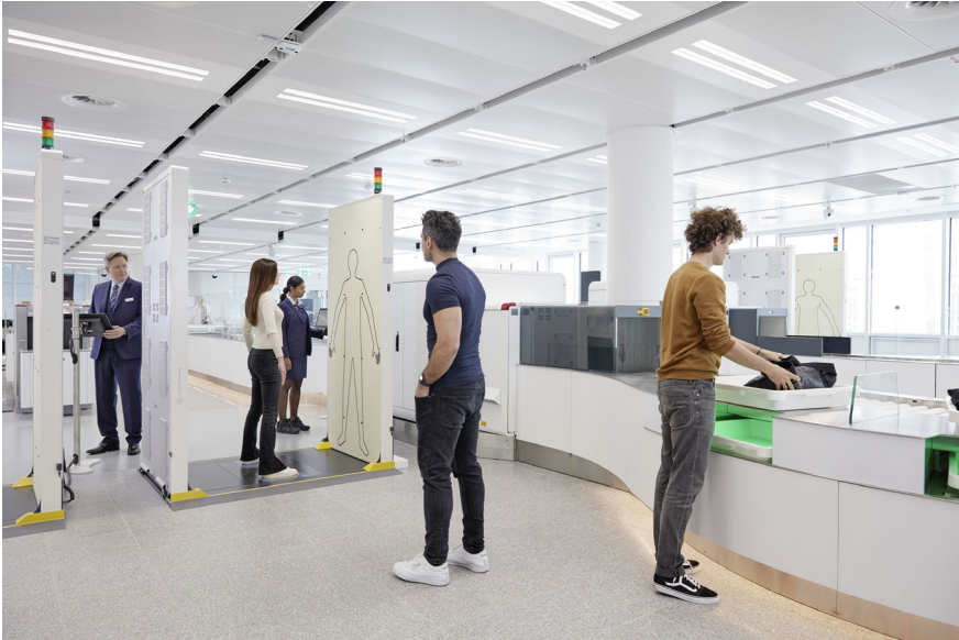
Fig. 2.3 Body scanner R&S®QPS201 from Rohde & Schwarz at Munich Airport. The scanner at 70 - 80GHz with more than 12000 antennas enables the detection of potentially dangerous objects hidden under clothing. Image source: Rohde & Schwarz
