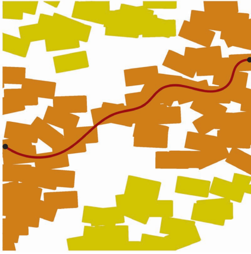
Figure 1.6: A percolating cluster of connected components spans the whole system and connects opposite edges; for an infinite system percolation is a geometrical phase transition.
