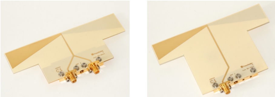
Figure 6.13.: Picture of the implemented “amplitenna” (CMCD PA C1)
