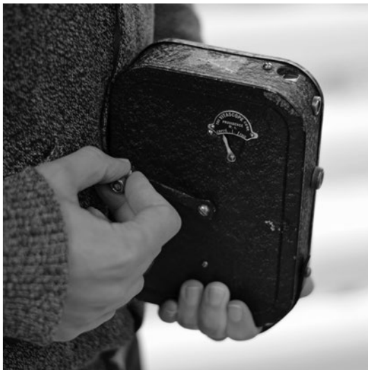
Fig. 12: Filming position of the Vitascope Movie-Maker.
