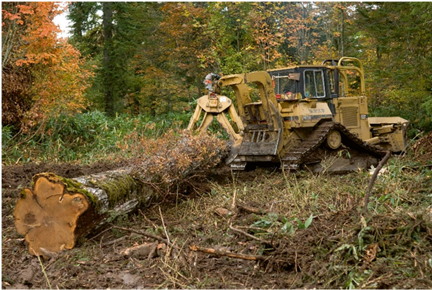
Fig. 9.2 Transportation of a trunk by a D4HTS grapple skidder (Shin Caterpillar Mitsubishi Ltd.) in Compartment 90, 2007. (Photo by the UTHF, licensed under CC BY-NC-ND 4.0)
