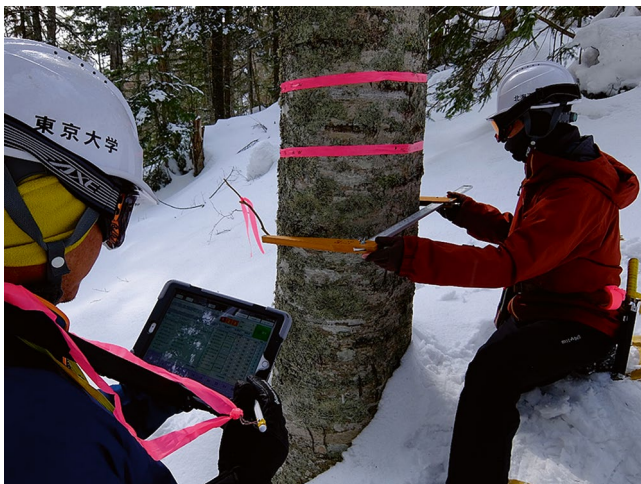
Fig. 8.10 Inventory plot survey conducted using a tree caliper and a tablet terminal. (Photo by Kota Kimura, used with the UTHF's permission, licensed under CC BY-NC-ND 4.0)
