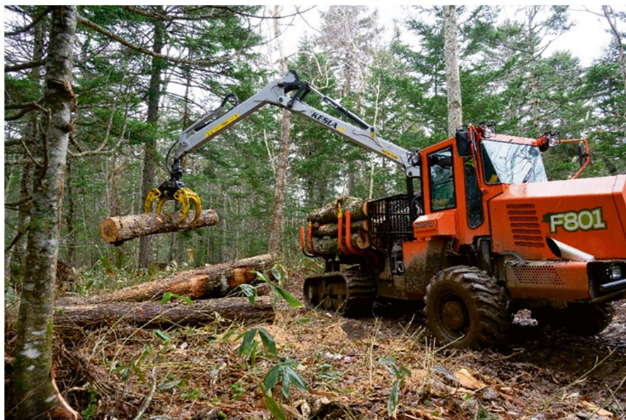
Fig. 9.3 Log transportation operation using an F801 Forwarder (Kato Works Co., Ltd.) equipped with a grapple crane (Kesla Oyj, Finland). (Photo by the UTHF, licensed under CC BY-NC-ND 4.0)
