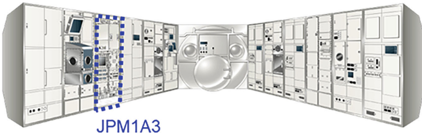
Fig. 4 Location of Ryutai Rack in JEM pressurized module (JPM1), Aft3 position (A3). This figure shows the interior view from the entrance side of JEM. The deck and ceiling side are not shown (©JAXA with permission)
