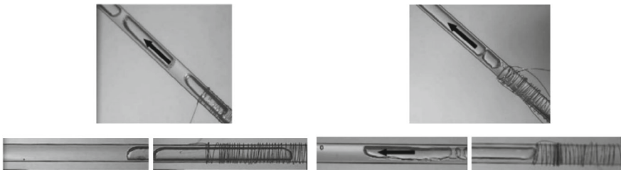
Fig. 16 Slug boiling behaviour in water (left) and SRWF (right) under different inclination with respect to the gravity vector. Reprinted from Savino et al. [78] with permission from Elsevier. All rights reserved
