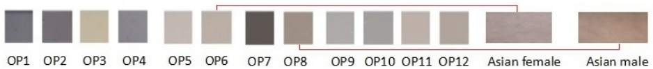
Figure 23: The correspondence of the color tone between the elastofluidic phantom matrices and the skin of the asian male/female volunteers is shown. The PVCp slabs in different color and the skin sites at the forehead of the chosen human volunteers are indicated.
