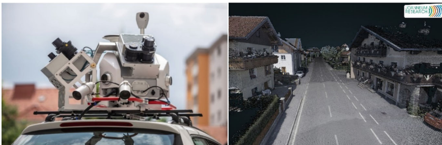
Fig. 1 Leica Pegasus 2 ultimate mobile mapping system (left), Colorized 3d point cloud (right). Source Joanneum Research
