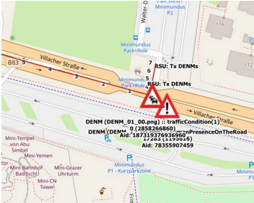
Fig. 6 Warning messages of cars and pedestrians crossing, issued and broadcasted upon detection by the awareAI based system. Source Modified from OpenStreetMap
