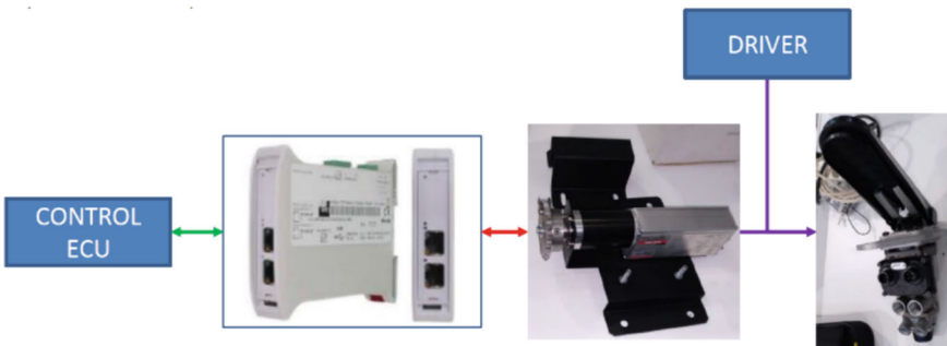
Fig. 5 Brake pedal control schematic for the I2EBAR bus. Source Authors' picture
