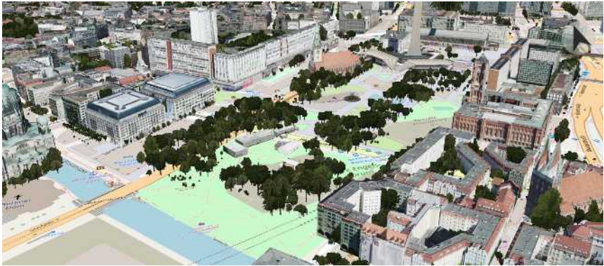
Figure 1.3: Alexanderplatz, Berlin, Germany. Virtual model based in CityGML with 3D buildings enriched by valuable meta information with regards to auralisation, like traffic lanes.
