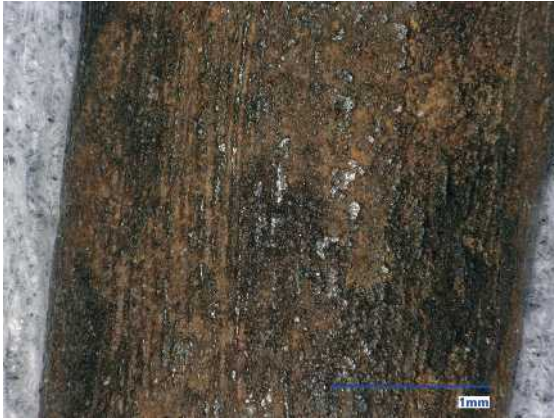
Figure 6.2. 3D microscope image showing surface striations on GR.5i.1939 (© The Fitzwilliam Museum 2023).
