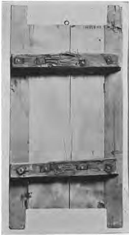
15. Wooden Mould for Making the End Plate of a Five- or Six-Plate Stove.
