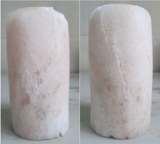
Fig. 2.13 Specimen failed in the uniaxial test
