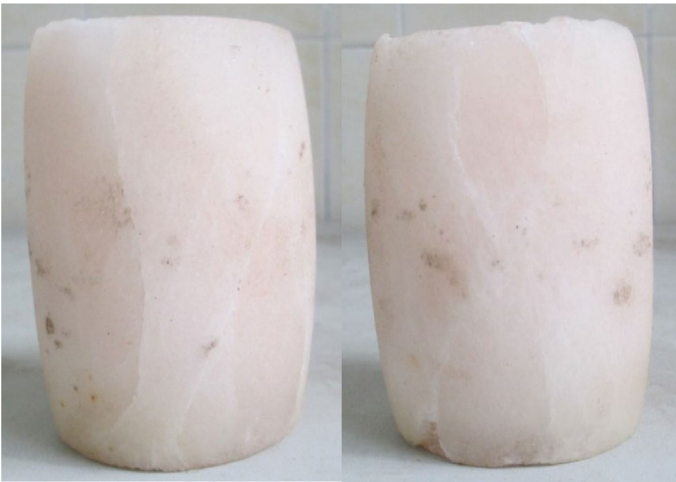
Fig. 2.21 Fractured rock salt specimen after D point from trial tests
