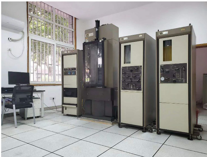
Fig. 2.6 The MTS 815 rock mechanics test system used in this experiment
