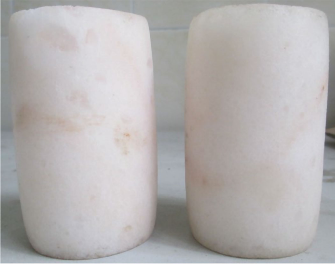
Fig. 2.20 Deformed rock salt specimen before D point from trial tests
