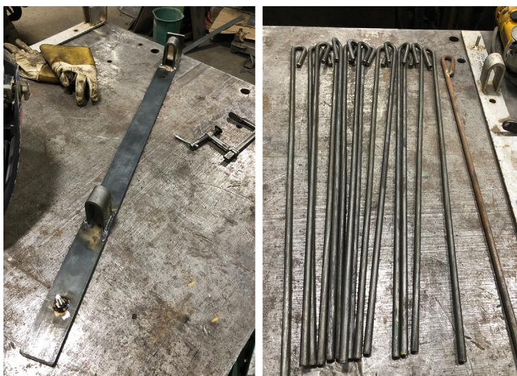
Fig. 11.5 One of the hog-pen brackets that I made (left) and pins for the brackets (right)
