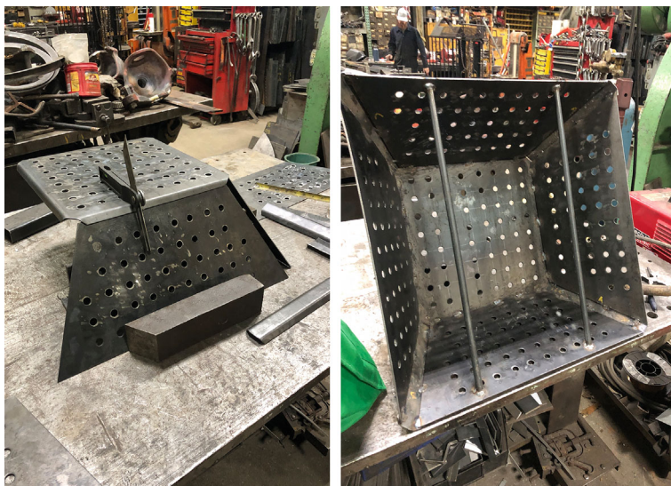
Fig. 11.7 Starting to fixture the drain basket (left) and the nearly finished drain basket (right)
