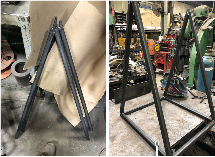
Fig. 4.2 My mistakes on the bank-sign angles (left) and the bank sign with correct angle joints (right)
