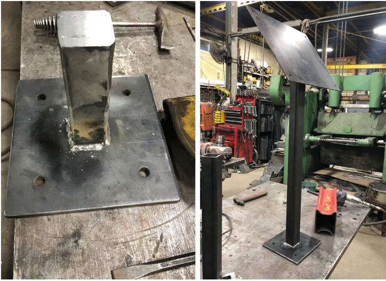
Fig. 11.6 The ground-down square-stock stand for the park sign (left) and the completed sign for the park (right)
