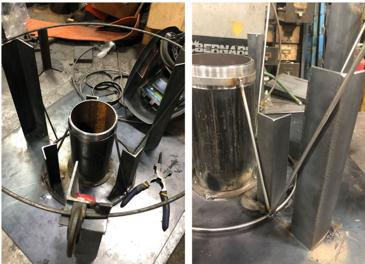
Fig. 8.7 The fixture that Jim designed for my lampshade skeleton project. On the left, the fixture holds a steel lampshade skeleton. I made it as a prototype for the client before switching to stainless steel. On the right, the fixture holds an incomplete stainless-steel lampshade skeleton
