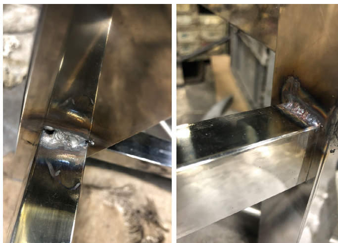
Fig. 4.6 The hole I burned in the chrome-plated chair (left) and my successful tig weld on the same chair (right)
