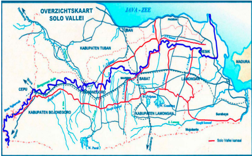
Figure 9.1: The Solo Valley Public Works project in the downstream portion of the Bengawan Solo. Source: Balai Besar Bengawan Solo, 2009
