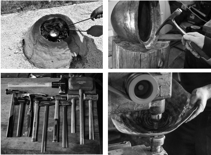
Figures 4.7a–d Experimental archaeology in the construction of a Negau helmet. (a) Melting bronze in a temporary furnace; (b) Shaping the Negau helmet; (c) Hammers used to shape the Negau helmet; and (d) use of a pneumatic power hammer to stretch the initial bronze sheet to c. 1.5 mm.
