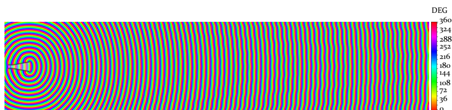
Figure 2.12: Phase of the electric field of the propagating wave radiated from the antenna. The phase fronts can be clearly identified as a regular pattern that helps to detect the direction of propagation.
