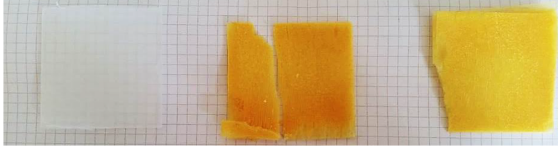
Figure A.10: Polypropylene plates without an additive (left), with 2 wt% C_{18}PEO_{10} (center) and with 2 wt% C_{18}PEO_{20} (right) stored for approximately 350 hours at 80 °C. Discolorization of the samples indicates significant degradation phenomena.
