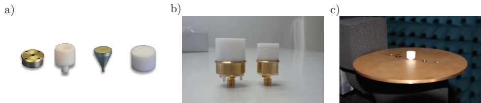
Fig. 8.6: a) Individual parts, b) manufactured prototypes and c) measurement setup of Monocone antenna. Note the size difference between the MCB element shown on the left side of b) and the MCA element on the right.
