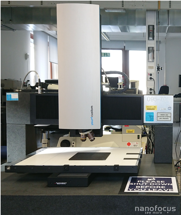
Fig. 3.7. Confocal laser-scanning microscope μsurf custom of the supplier NanoFocus.
