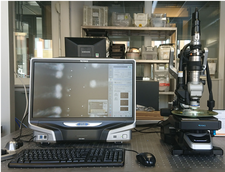
Fig. 3.3. Digital microscope VHX-6000 of the supplier Keyence .
