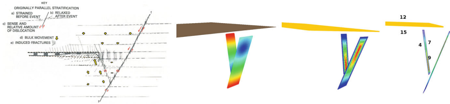
Fig. 6.53 Strike section through a slope showing a double source mechanism conceptualised by Ortlepp ( first ). Rupture history of the Ortlepp source, with initiation time per point obtained from radial distance from the focus ( second ). Slip history of the Ortlepp source, with final displacements determined by a k -square distribution ( third ). Synthetic sensor placement around the fault-stope corner ( forth )
