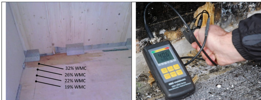
Fig. 13. Horizontal gradient of moisture content in CLT, example of handheld measurement device (Senzomatic.com)
