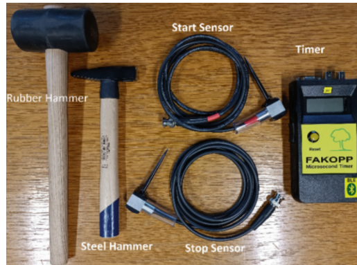
Fig. 1. FAKOPP microsecond timer
