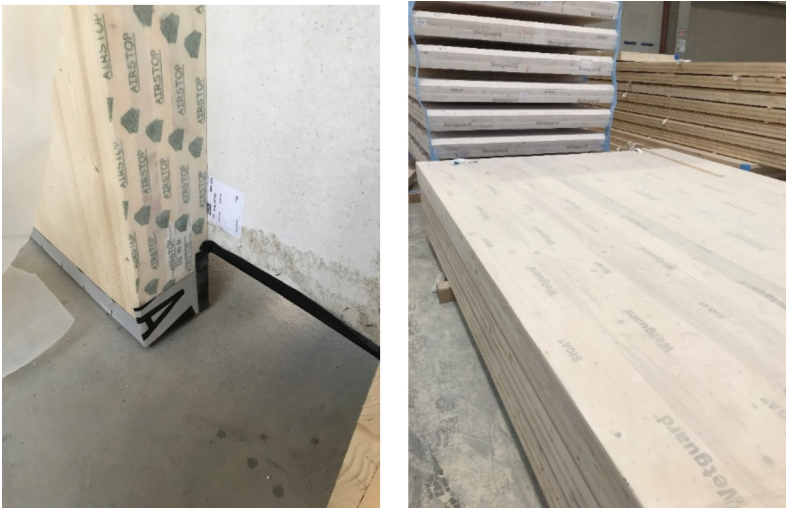
Fig. 8 Left – Factory-applied tapes and membranes for end-grain protection. Right – Factory-applied self-adhesive membrane for CLT face protection.
