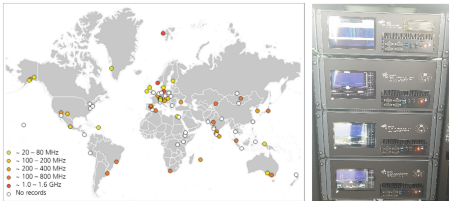
Fig. 2. Global distribution of CALLISTO receivers colored by frequency (left), and compact receivers of GIFDS, L-Band-, VHF/UHF-, and HF/VHF-CALLISTO (from top to bottom, right).
