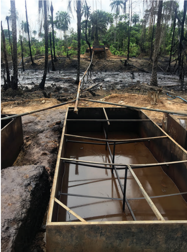
Figure 9.1. Tanks at an artisanal refinery, connected to a cooking pot where kerosene, gasoline, and diesel are refined. Photo by Omolade Adunbi.
