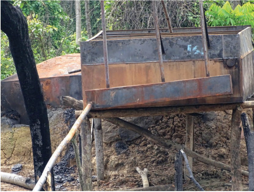
Figure 9.2. Cooking pot in an artisanal refinery. Crude oil is poured into the pot that sits on top of a molded platform with fire underneath the platform. The pots are connected to different tanks within a radius where gasoline, diesel, and kerosene are refined. Photo by Omolade Adunbi.
