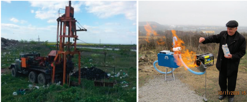
Figure 5.1 Research of flow rate and gas content of the well.
